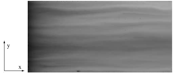
Figure 6. Greyscale map of the normalized local transit time \bar{t}(x, y)U/x . Flow is from left to right. Dark (resp. light) regions correspond to locations where \bar{t}(x, y)U/x < 1 (resp. \bar{t}(x, y)U/x > 1 ). Mean flow velocity U = 0.014 \text{ mm/s} ( Pe = 150 ), polymer concentration 1000 ppm).
