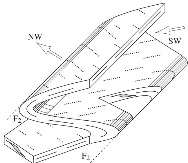
**Figure 8.** Interpretative diagram showing how secondary (F<sub>2</sub>) folding of the foliation and lineation may produce locally apparent top-to-the-SW shearing.
