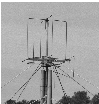
Fig. 3: Array n°3 of eight HF collocated antennas (patent n°99 16112)
