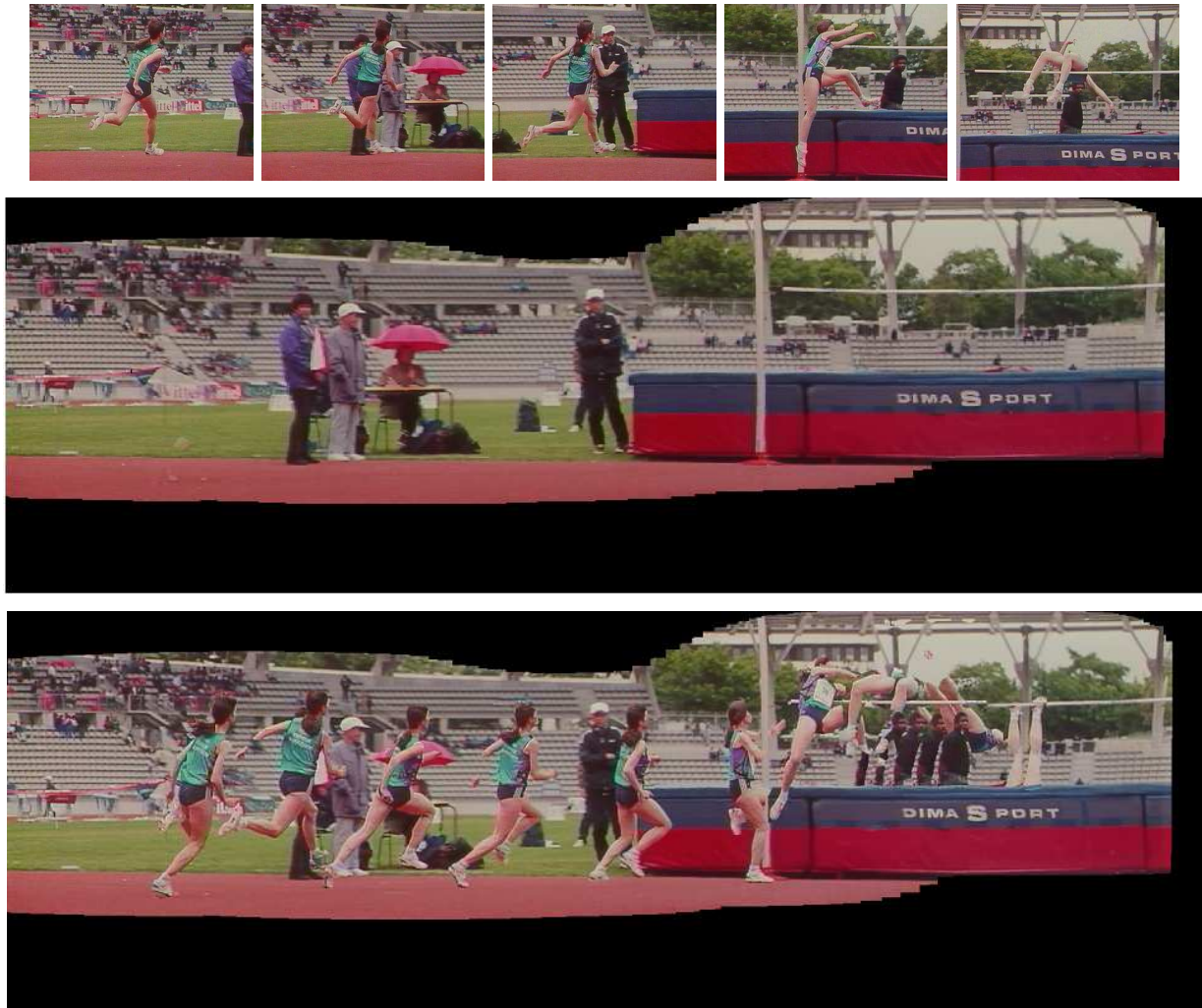
Figure 1: This figure shows 5 images extracted from a 350-frame sequence (top), the static panorama or the background image (middle) showing the static objects used to estimate the time-varying camera parameters (focal length, pan and tilt angles), as well as the motion panorama showing a high-jump athlete in various postures as it would have been filmed with a wide-angle static camera (bottom). Notice the fine image resolution associated with the output images.
