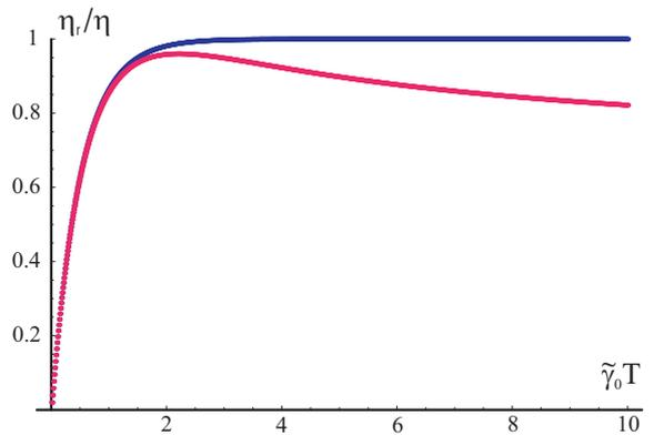
FIG. 4: (Color online) Readout efficiency  $\eta_r$  (normalized by the *cw* efficiency  $\eta$ ) versus pulse “area”  $a(\infty) = \tilde{\gamma}_0 T$  when the LO is either the retarded readout pulse (lower curve) or a pulse temporally matched with the atomic emission (upper curve).
