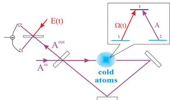
FIG. 1: (Color online) Quantum memory set-up: field  $A^{in}$  is sent into a cavity containing an ensemble of three-level atoms. The coupling of the intracavity field  $A(t)$  with the atomic ground state variables is dynamically controlled by a pulsed coherent field  $\Omega(t)$ . The fluctuations of the output field  $A^{out}$  are measured by homodyning with a local oscillator  $E(t)$ , the temporal profile of which may be adjusted so as to optimize the detection efficiency.
