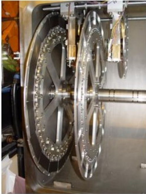
Figure 1: Target chamber with the two wheels bearing 18 Pb or Bi targets and 18 carbon charge equilibration films.
