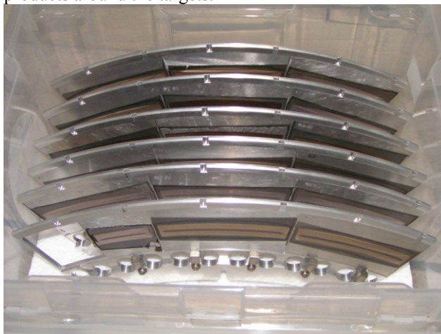
Figure 4: ^{208}\text{Pb} targets on segments of the wheel after irradiation.
