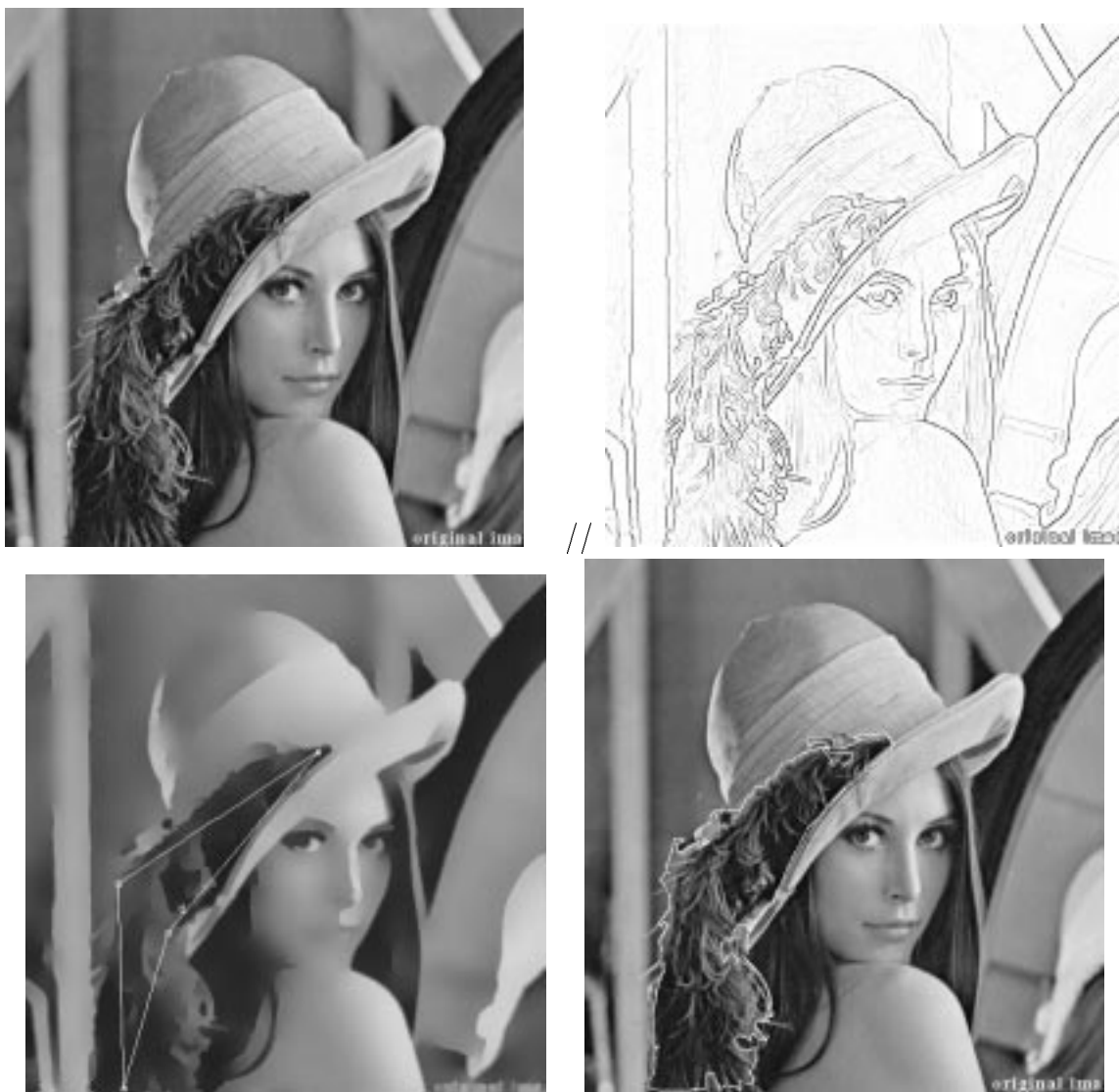
Fig. 7. Lena image. From top to bottom and left to right: the original image ( 512 \times 512 ), the Canny-Deriché gradient image ( \alpha = .35 ), the snake-spline initialization on the diffused image (100 iterations, \beta=6 \text{ E-}05 , s=5 and time to calculate equals 245 secondes), and the snake spline result with ( sp=3 , b=1 , sm=0 ).
