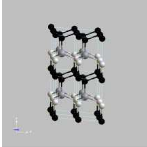
Figure 9.5: Crystal structure of the trigonal III-BC 2 N phase.
